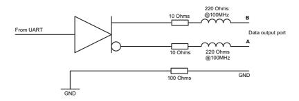
Figure 60 Data output port schematic
