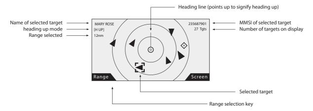
Figure 12 Target plot screen
