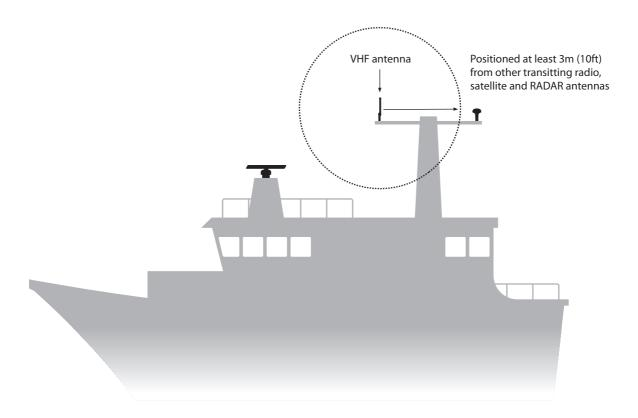
Figure 41 VHF antenna installation
