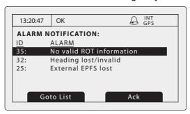
Figure 16 Alarm notification screen
