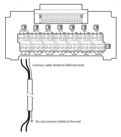
Figure 46 Connecting data interface cable shields
