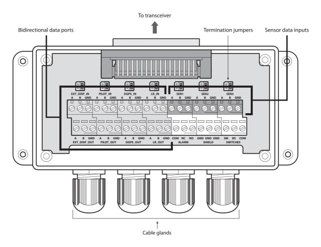
Figure 44 Junction box connections
