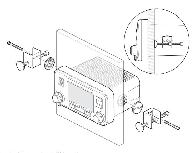
Figure 36 Panel mounting the AIS transceiver
