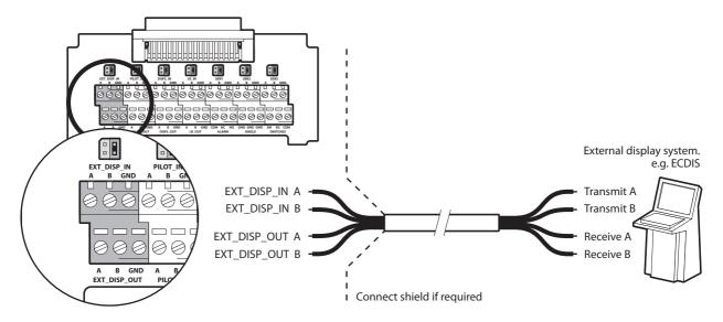
Figure 45 Example connection to external display equipment
