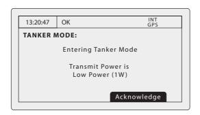
Figure 30 Tanker mode entry acknowledgement screen
