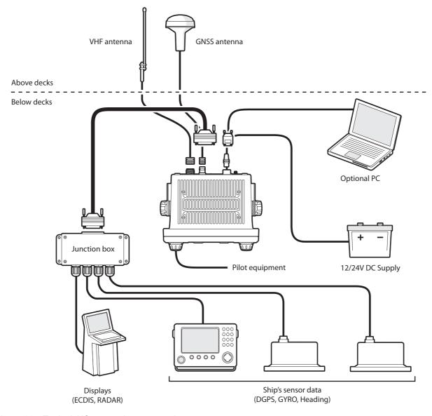
Figure 32 Typical AIS transceiver connection
