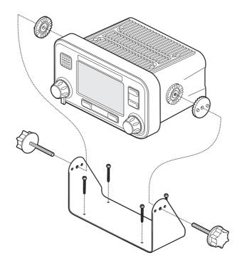
Figure 35 Mounting the AIS transceiver
