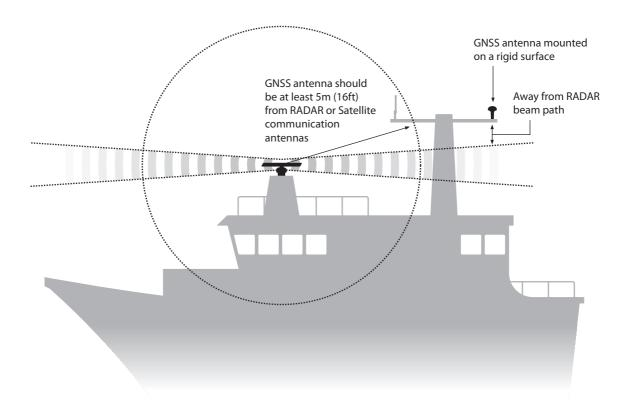
Figure 39 GNSS antenna location
