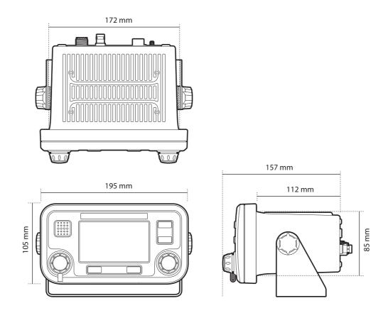
Figure 34 AIS transceiver dimensions
