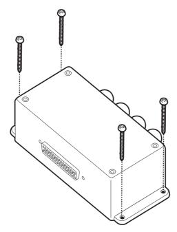
Figure 38 Mounting the junction box
