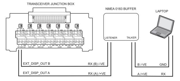
Figure 49 Single ended input connection
