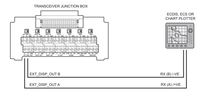
Figure 48 Differential input connections
