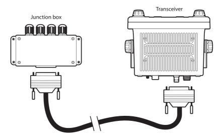
Figure 43 Connecting the junction box to the transceiver
