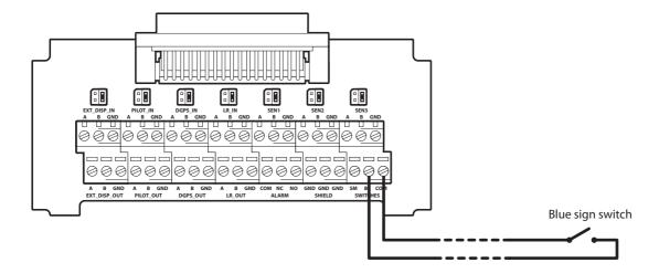
Figure 58 Blue sign switch connection
