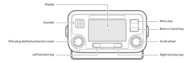
Figure 2 Transceiver front panel
