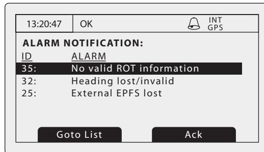
Figure 16 Alarm notification screen
