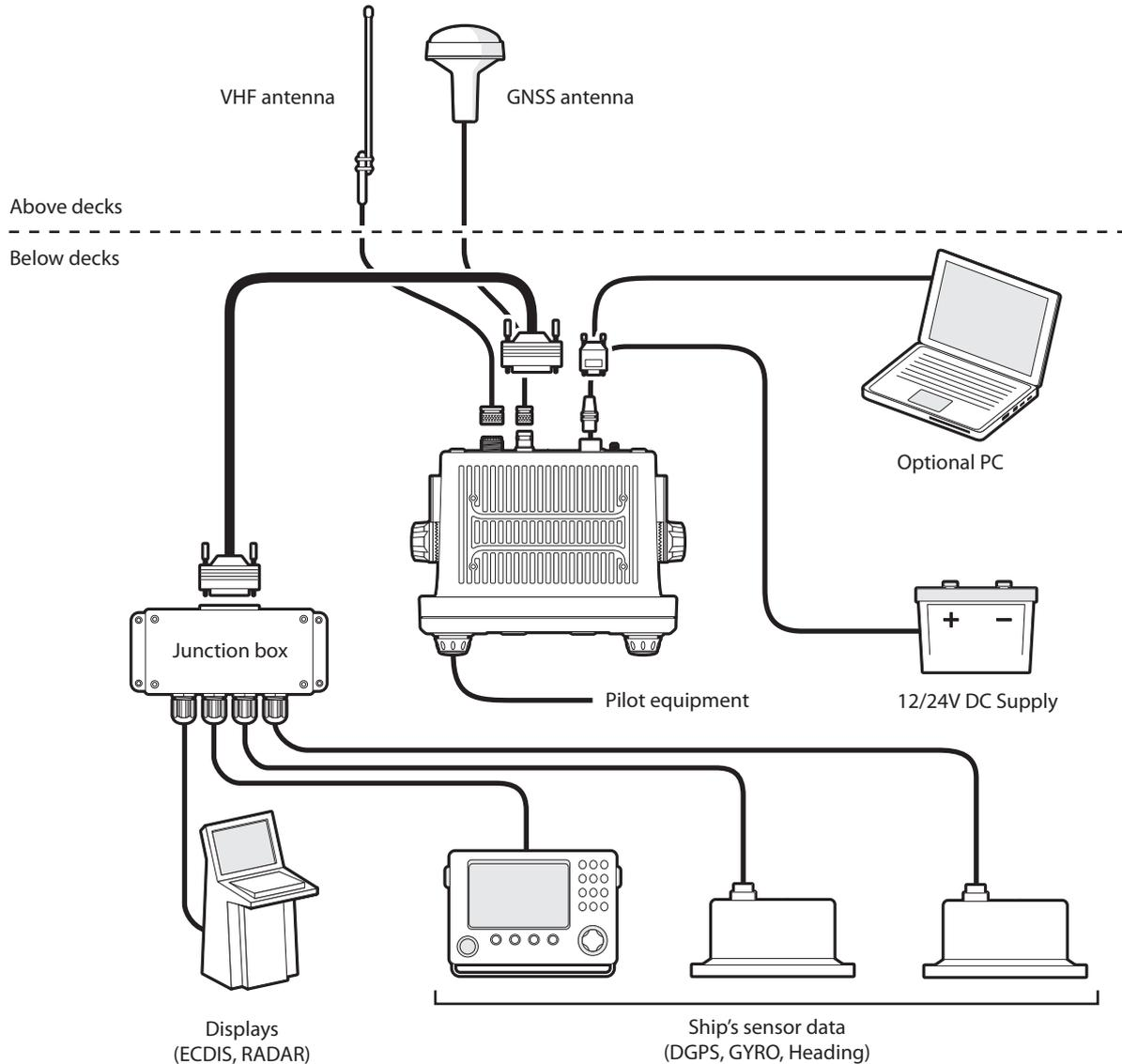
Figure 32 Typical AIS transceiver connection
