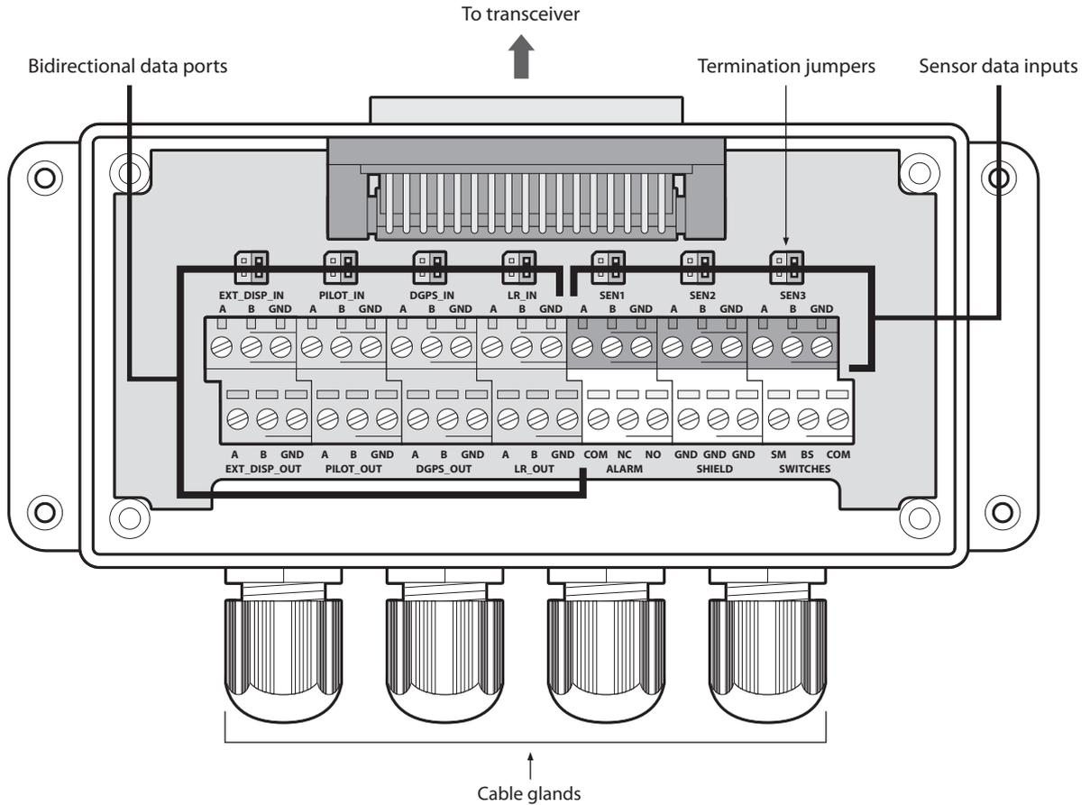
Figure 44 Junction box connections
