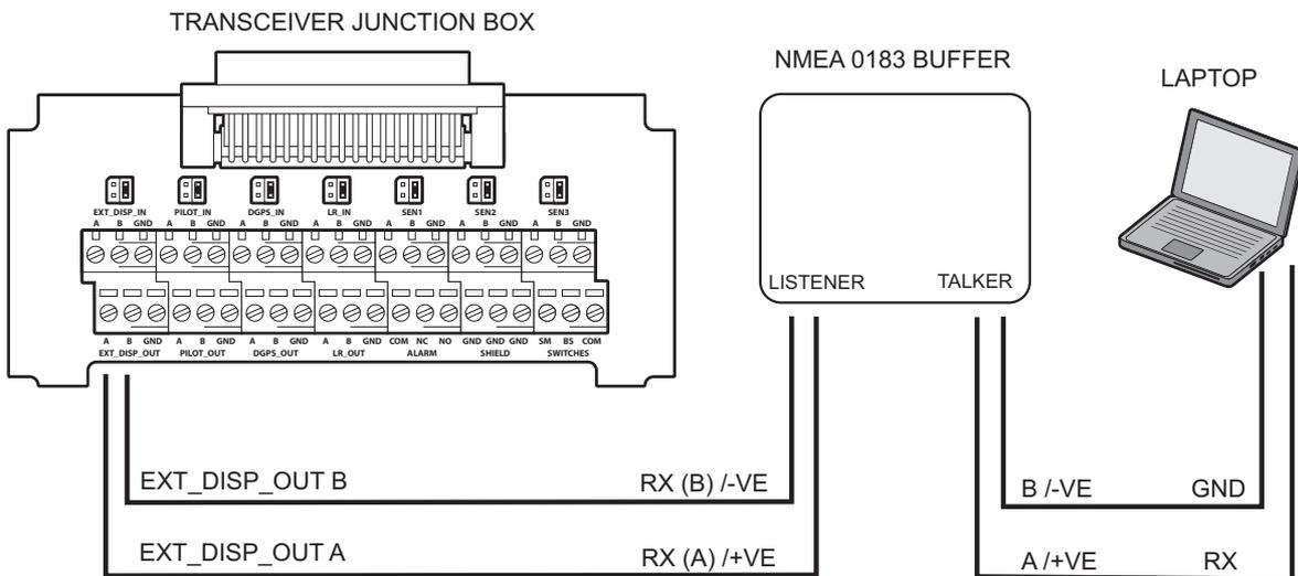
Figure 49 Single ended input connection
