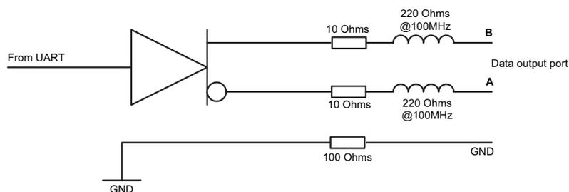
Figure 60 Data output port schematic
