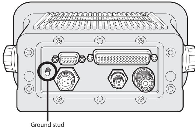
Figure 51 Grounding the transceiver
